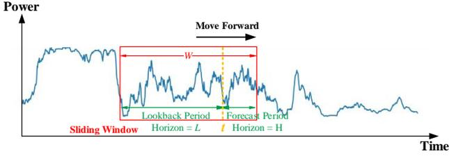
FIGURE 3 Sliding window of signals.
